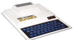
The ZX-80 was designed with only the base necessit the shelf components - there are no custom or propri involved.
